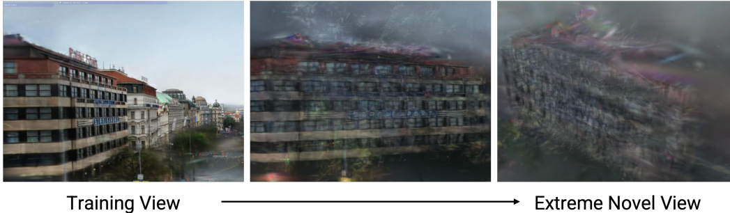
Figure 2. Example of Gaussian splatting artifacts at extreme novel views. The building’s visual quality deteriorates significantly when the camera orbits from a training view (left) to an extreme novel view (middle and right).
