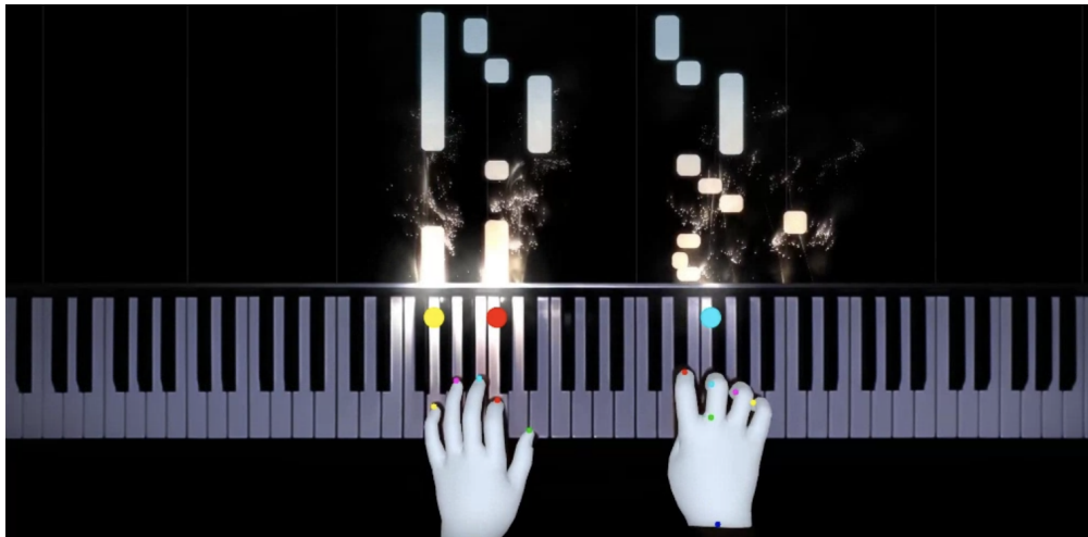
Figure 7: Example of automatic fingering labeling. The small colored circles on each hand denote the estimated location of each fingertip, and the large colored circles on specific keys denote that the corresponding finger should press that key. In this example, the right thumb is in the middle of a finger crossing motion and appears directly underneath the middle finger. The automatic labeling correctly assigns that key to the right middle finger.
